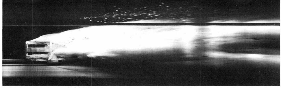
IMAGE MOTION photograph stops accelerating rocket sled as it emerges from a simulated explosive debris cloud. The wedge-shaped nose contains
